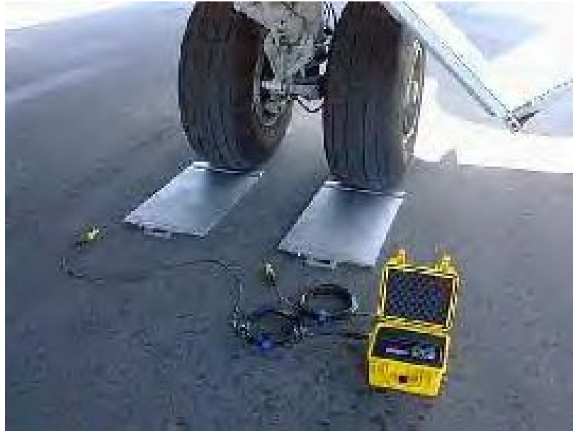
40,000 lb low profile pad with digital indication
